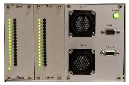
The standard configuration for the Functional Tester consists of 32 flexible channels with 2x 37 pin mass interconnects for Power and loads and 2 DSUB9.
